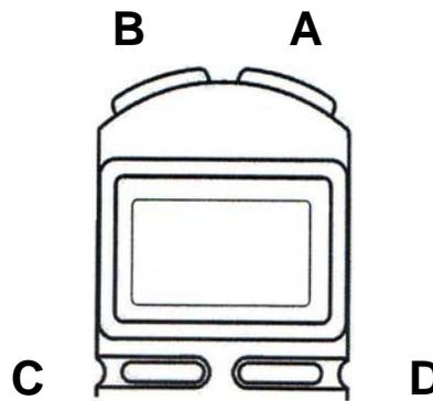
The **SC-505W** is a Multi-Mode Stopwatch featuring single event timing, interval (LAP) chronograph or accumulated (SPLIT) chronograph functions. You can time events in any mode up to 24 hours with 1/100 second resolution. The SC-505W automatically counts up to 199 lap or split readings and has memory recall of the last twelve (12) readings.
