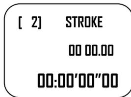
A stroke rate is determined by measuring the time it takes to complete a certain activity or set of actions and then calculating how many times that it will be completed in one minute. For example, if a swimmer completes three (3) strokes in 10 seconds, then the Stroke Rate Calculator will read 18 strokes per minute.
