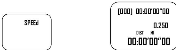
The Speed Timer will not operate unless the Chronograph is stopped and Reset to all zeros. STOP indicator will appear.
