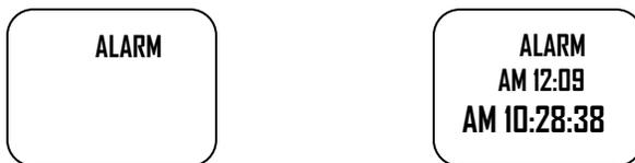
While in ALARM TIME mode, press and hold “F” for 2-3 seconds. SET indicator appears. Alarm hours will begin flashing. Advance Alarm Hours by pressing or holding “A”. After setting Alarm Hours, Press “B”. Alarm Minutes will appear flashing. Advance by pressing or holding “A”. The alarm will automatically be armed (set to go off) after the Alarm Time is adjusted.
