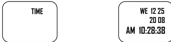
To begin the setting process, press and hold “E” until Seconds begin to flash and SET appears in the upper row of the display.
