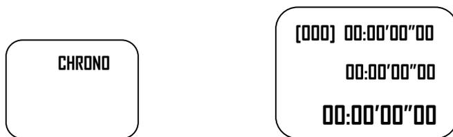
The “stopped” chronograph (stopwatch) display will appear as shown above. If not, press “A” to stop and “B” for 2-3 seconds to reset the display to all zeros.
